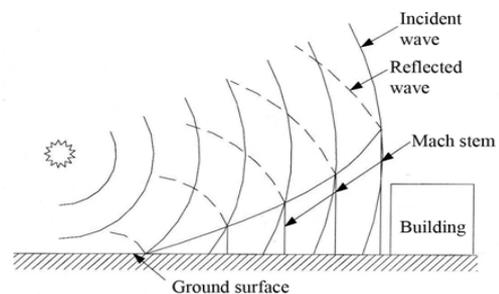
Fig 1: Air burst explosion
