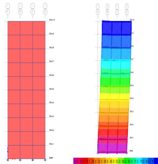
Fig 9. Model and displacement in mm of frame with 0.115 m thick infill wall for 2500 kg TNT
