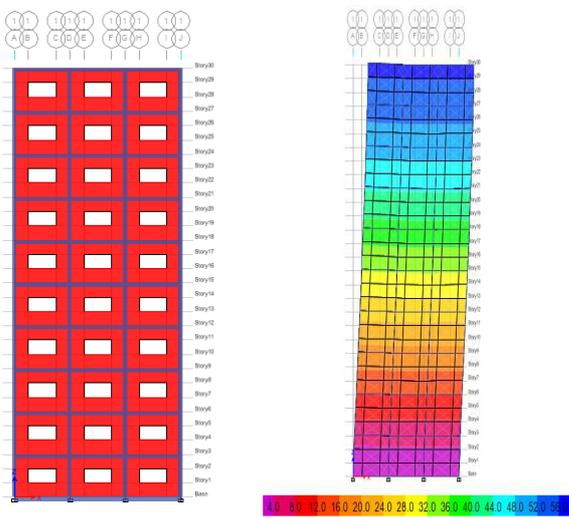
Fig 10. Model and displacement in mm of frame with 0.23 m thick infill wall with opening for 2500 kg TNT
