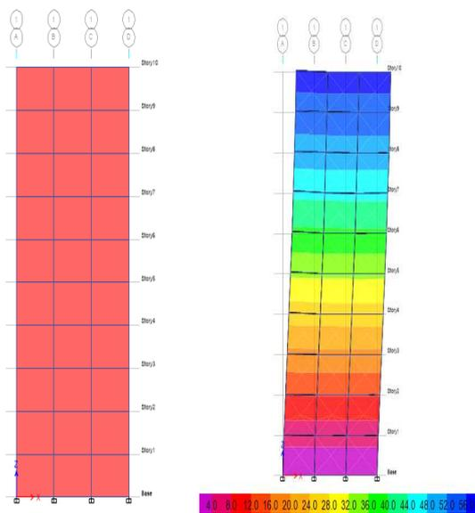
Fig 8. Model and displacement in mm of frame with 0.23m thick infill wall for 2500 kg TNT
