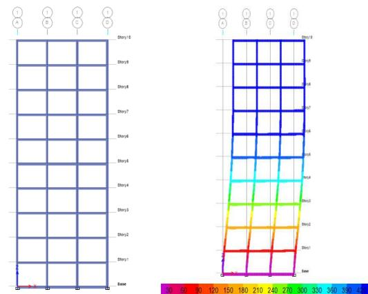
Fig 7. Model and displacement in mm of bare frame for 2500 kg TNT
