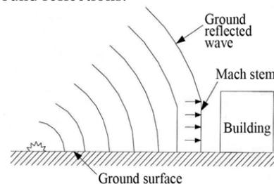
Fig 2: Surface burst explosion
