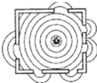
Fig 4: Fully vented explosion
